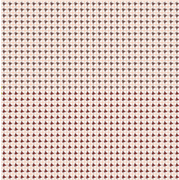
Figure 16: Mass setup for topological waveguide. Two lattices reflections of one another are sandwiched.
